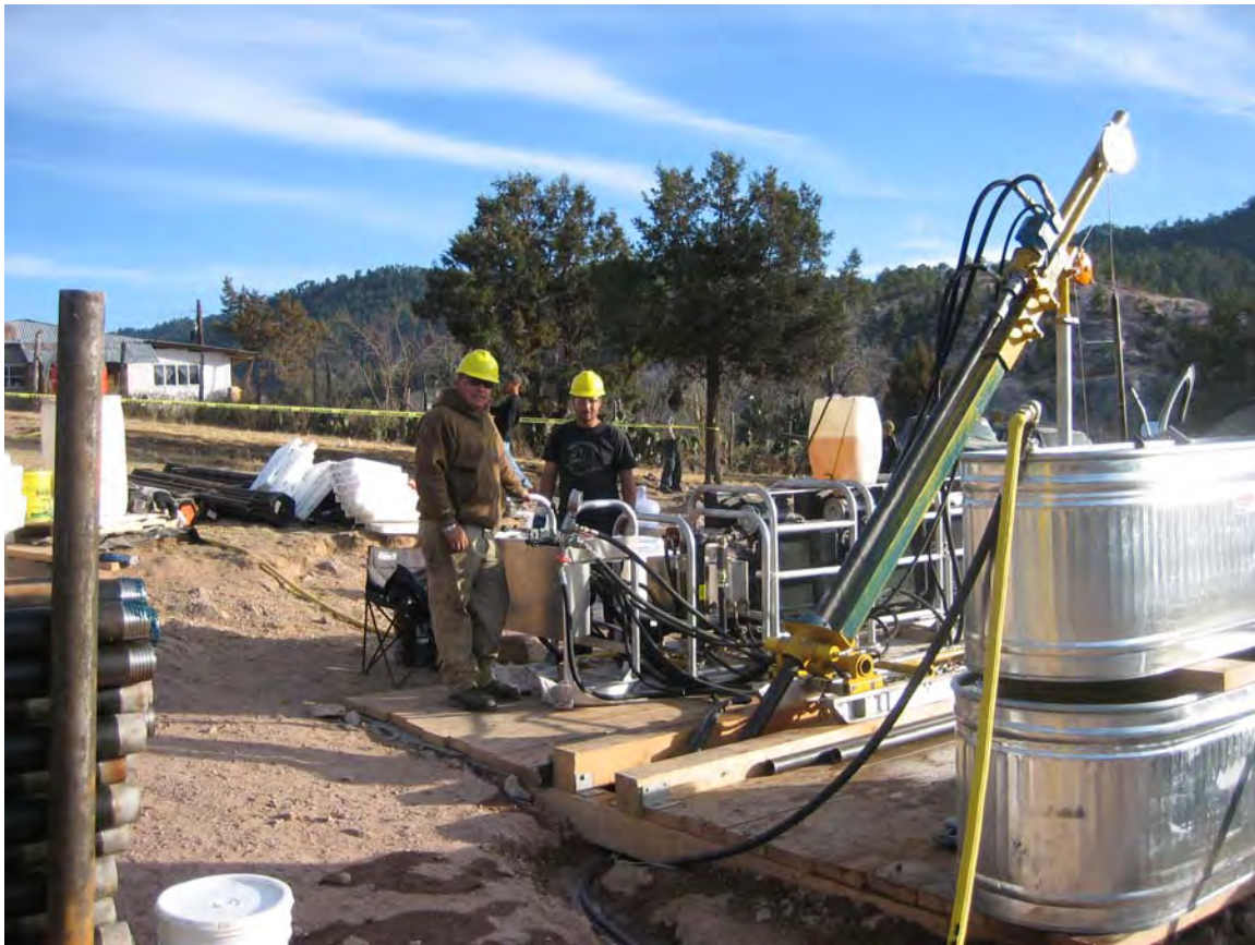
Photo 13.1 Hydracore Gopher Drill at Drill Hole LBDDH-001
