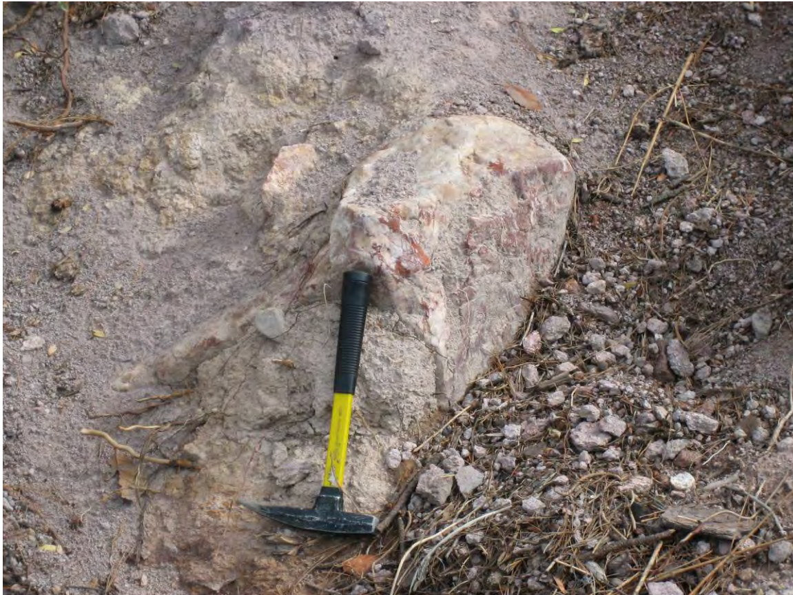
Photo 9.1 Quartz vein cobble at contact between LVG and UVG rocks. Head of hammer is in weakly argillic and Fe stained andesite tuff (LVG) while gray color rock above handle is quartz-biotite rich crystal tuff (UVG)
