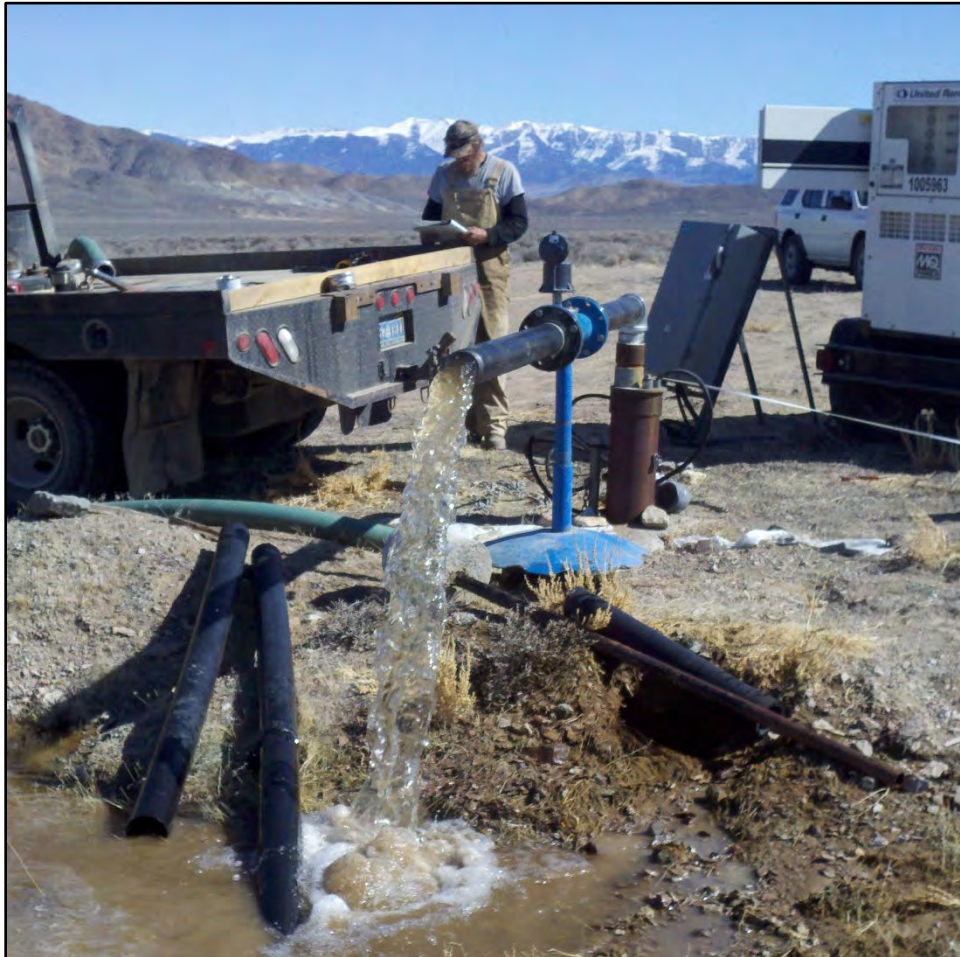
Figure 18.1: Photo of Water Well during Pump Testing
